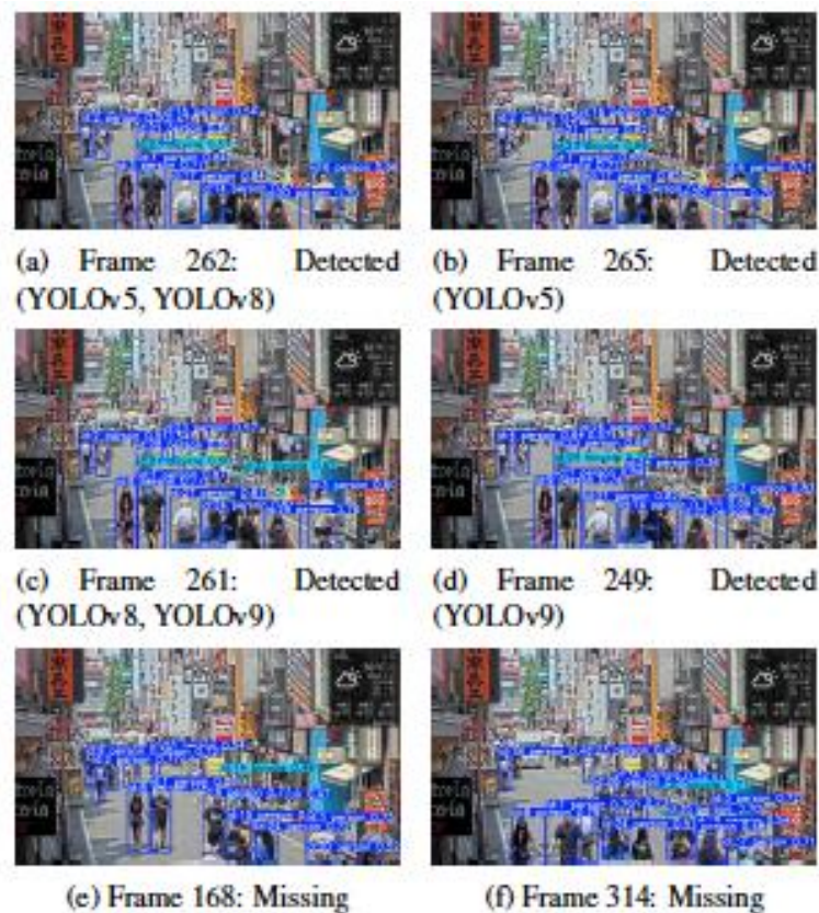
Figure 7 Detected and Missing Frames in the YOLOv5 Model. (Kabukicho Live Channel 2, 2022)
